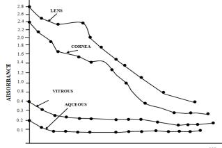
300 320 340 360 380 400 450 500 550 600 650 700 750 800 850 900 950 FIG. 1: Plot of Absorbance against Wavelenght in mm.
